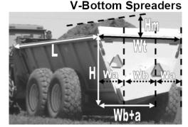
feet, so multiply the weight of the five gallon bucket by 1.5 to convert gallons to cubic feet and follow the formula below to calculate the capacity of the spreader in tons:
