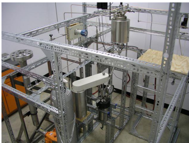
Figure 4. Continuous hydrothermal process reactor system. (Ocfemia et al., 2006)
